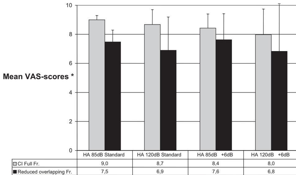
Fig. 6. Mean scores on the visual analogue scale (VAS) are shown for each test condition. The error bars represent standard deviations.
